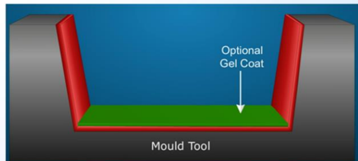
Basic Process of Hand Lay-up
